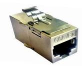
Shielded Inline Coupler, C6A avoids the need for rear termination and allow two patch cables to be connected directly, no tools required. This standard keystone jack fits any keystone wall plate, Patch panel, or surface mount box. Rated for Cat6A network this jack allows for bandwidth up to 10Gigabit per second.
